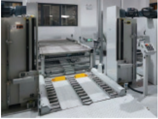
Hydraulic truck handling + connecting lifting machine (without pit)
